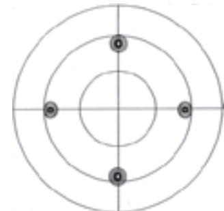
Fig.1 (111) pole figure for first CeO 2 layer deposited on Ni-5at%W substrate (Δφ=5.8°).
