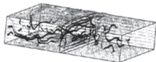
Fig.3 Example of simulation result. (Heat flux vector and its stream-line in case(2))
