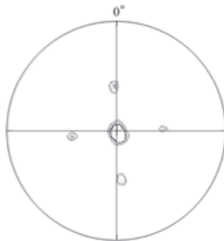
Fig.2 X-ray (103) pole figure of the YBCO deposited on the \text{CeO}_2/\text{YSZ}/\text{CeO}_2/\text{Ni}/\text{Cu} substrate
