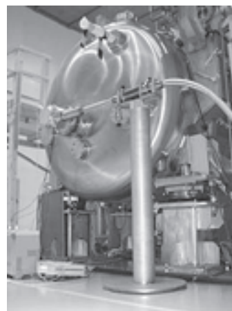
Fig.1 A 14T Superconducting split magnet in operation with a cryogenic probe for 600MHz NMR spectrometer
