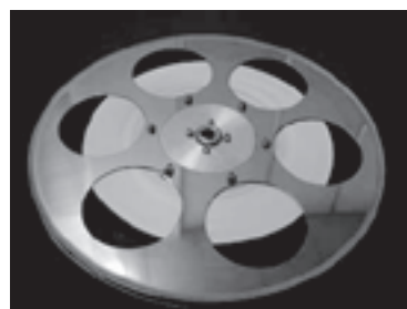
Fig.1 Appearance of 500m-GdBCO tape
