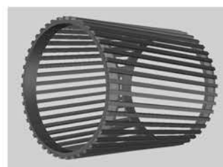
Fig. 1 Schematic diagram of a squirrel-cage rotor winding.
