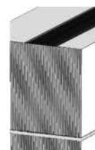
Fig. 3. Current distribution of Cu layer
