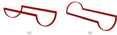
Fig. 3 (1) the arc section added to the end of the rectangular coil (2) one of the arc portions reversed.
