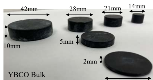
Fig.1 Photograph of superconducting bulk material for magnetic shielding
