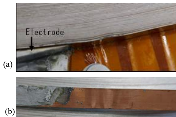
Fig.2 Deformation of the outermost turn near the electrode of the lower pancake coil of M1U.
