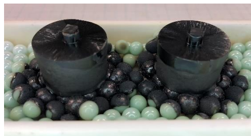
Fig.1 Appearance of SmBCO bulk after crystal growth
