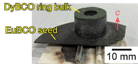
Fig. 1. Photograph of a SDMG processed DyBCO ring bulk grown on [001] oriented EuBCO seed plate.
