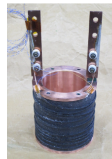
Fig.2 Photograph and the specifications of the MgB 2 solenoid coil fabricated with a 65m long IMD 7-filamentary MgB 2 /Cu wire.
