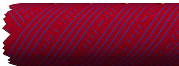
Fig. 2 Side view of an analyzed SCSC cable with 2.5-mm core diameter.
