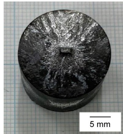
Fig. 1. Appearance of DyBCO melt-textured bulk grown from a Nd123 single crystal placed at the top surface.
