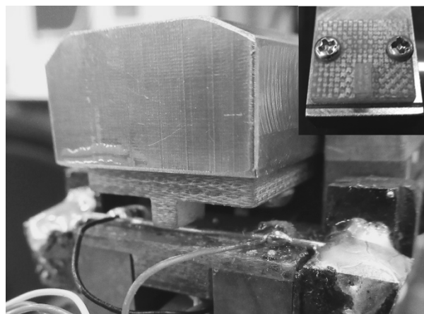
Fig. 1 The sample set-up on the critical current measurement with the transverse compressive stress.
