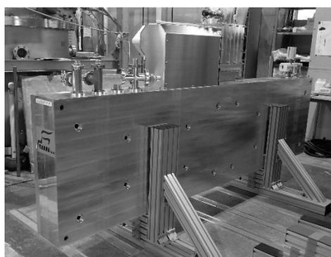
Fig.2 REBCO magnet for the electromagnetic vibration tests
