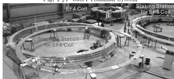
Fig.2 EF5 and EF6 Coil Manufacturing
