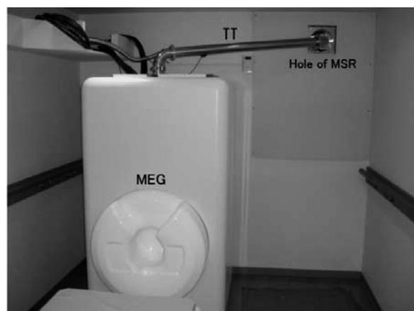
Fig.2 HCS installed on a commercialized MEG made by Yokokawa Electric Corporation Inc. (PQ1160C). TT: transfer tube, MSR: magnetically shielded room.
