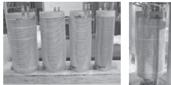
Fig. 1 Photo of the coil wound with REBCO tapes.
