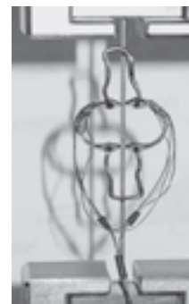
Fig. 2 Averaging dual extensometer system. Total mass ~ 0.6 g
