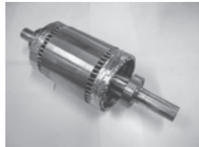
Fig. 1 Photograph of a squirrel-cage hybrid HTS rotor
