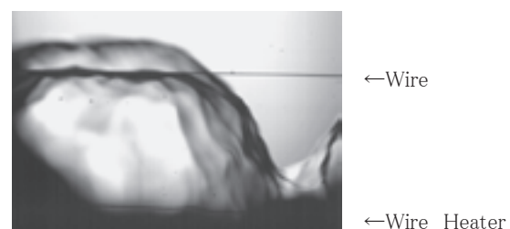
Fig.3 A visualization result of film boiling under micro gravity
