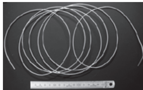
Fig. 1 The extruded 1mmφ wire of high-V f MgB 2 /Al composite material.
