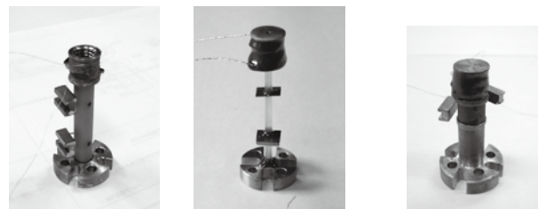
(a) AIN200 (b) Single crystal sapphire (c) Nitofix
