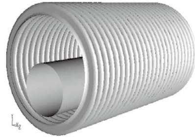
Fig. 1 A geometry of the bellows pipe; length is 150 mm, decentering is 15 mm
