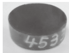
Fig.3 Bulk superconductor with resin impregnation
