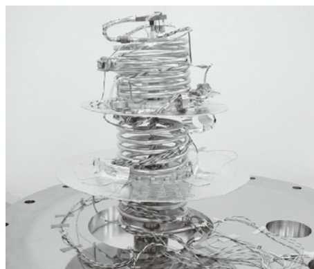
Fig. 1 Heat exchanger assembly with the orifice and the by-pass line
