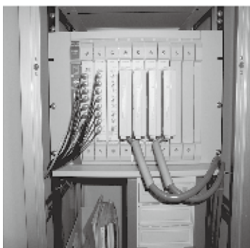
Fig.1 New data acquisition system for the normal-transition detection.
