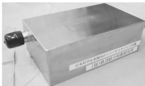
Fig.2. Newly developed cryostat that bulk superconductors entered
