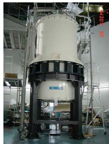
Fig. 1 Photo of the 1GHz-class NMR
