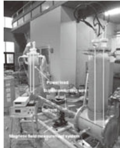
Fig. 1 Prototype DC superconducting cable for railway
