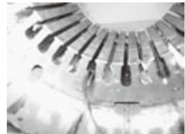
Fig. 1 Photograph of DI-BSCCO<sup>®</sup> (Type ACT) short sample in a slot of stator core.
