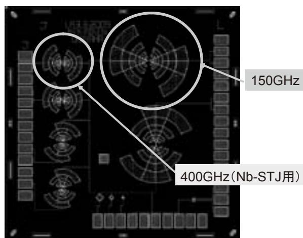
Fig.1 Design of an Antenna Coupled Al-STJ
