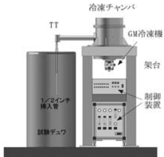
Fig.2 HCS with 1/2 inch insert tube for general superconductive apparatuses.
