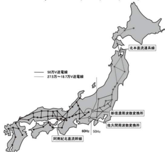
Fig. 2 The present main power grid of Japan. Left-hand side is 60Hz, and right-hand side is 50 Hz, and UHV DC is used at the connection part.
