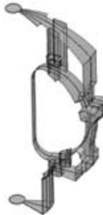
Fig.2 Overall 20 degree thermal shield
