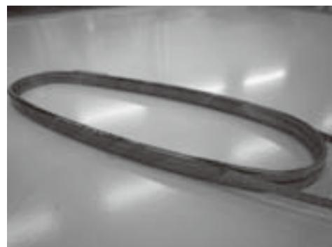
Fig. 2 Photograph of racetrack double-pancake coil made of DI-BSCCO<sup>®</sup> (Type ACT).
